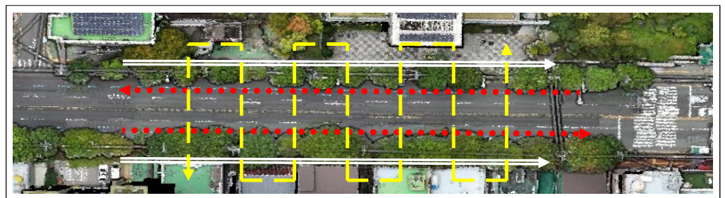
Figure 2. Lidar data collection path and method Legend: — Walking, ..... Vehicle, - - - Drone
